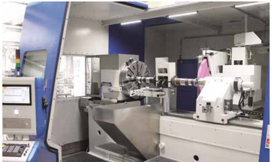
The AKP range for landing gear grinding machines with gap bed
