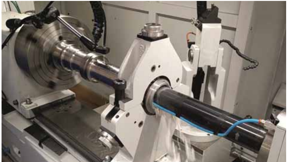
Different wheelhead configurations are available for internal grinding processes
