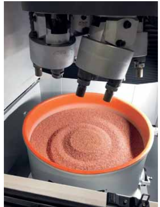
The processing bowl of the plug-and-play drag finisher can be easily exchanged with a fork lift truck. This allows quickly switching from one application to another without having to replace the processing media
