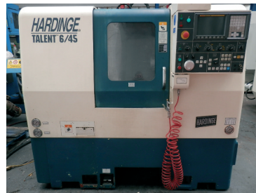
HARDINGE TALENT 6/45 CNC LATHE C/W FANUC CONTROL
