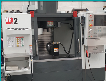
Haas VF2 vertical machining centre, New 2018, New 2018, HRT210 4th axis, high speed machining option, speeds to 8100rpm, 914 x 356mm table, X=762 Y=356 Z=508mm £P.O.A.
