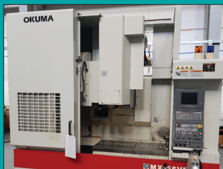
Okuma MV55 VB vertical machining centre, Ex Rolls Royce, Excellent condition, 1300 x 560mm table, BT50, 32 ATC, speeds to 6000rpm, X=1050 Y=560 Z=460mm capacity £P.O.A.
