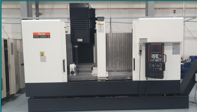
Mazak VTC 300C II vertical machining centre, New 2015, Mazatrol PC Fusion 640M, speeds to 12000rpm, Kitagawa 4th axis, BT40, 2000 x 760mm table, X=1740 Y= 760 Z=660mm capacity. £P.O.A.
