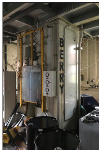
500 Ton Berry Hydraulic press complete with isothermic Bolsters/plattens.
