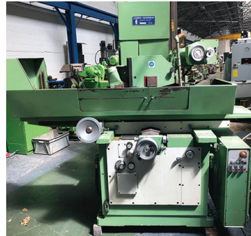
JONES & SHIPMAN 1415 GRINDER C/W MAGNET AND COOLANT
