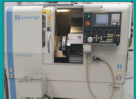
Hardinge Talent 8/52 CNC lathe, New 2006, Fancu OiT, 51mm spindle bore, 12 station turret, speeds to 5000rpm, VDI 30, 284mm max diameter, 381mm max length £P.O.A.
