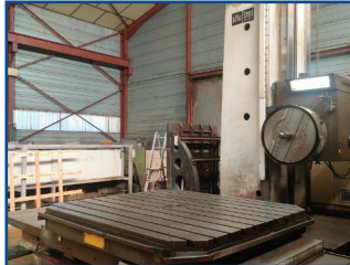
Union BFT 130 CNC Horizontal Borer Heidenhain 355 control
