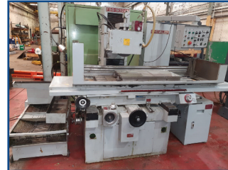
Chevalier 3 axis Automatic Surface Grinder Capacity: 810 x 405mm
