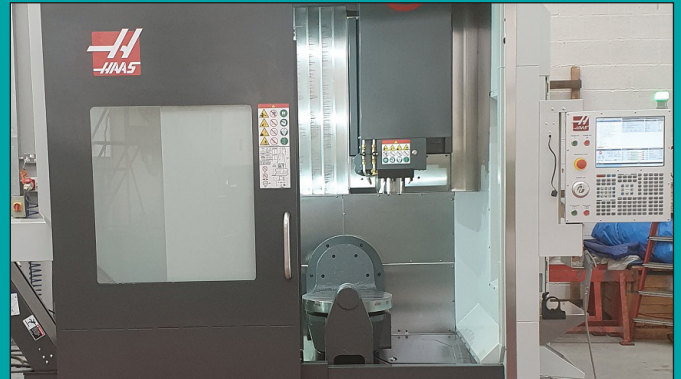
Haas UMC – 750 5 axis machining centre, New 2019, 90 hrs, Haas CNC, 500mm dia table, 12000rpm, probing, X= 762 Y=508 Z=508 C=350° B=110° to 35°. £P.O.A.
