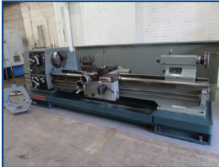
Colchester Magnum 1250 Gap Bed Lathe 2500mm between centres
