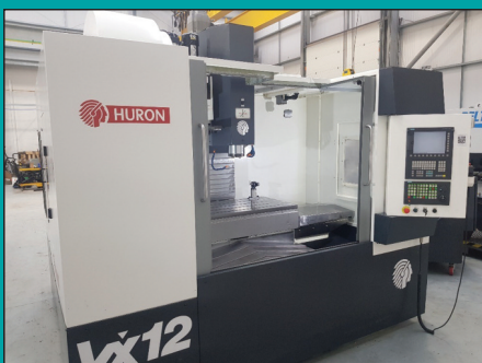
Huron VX12 vertical machining centre, New 2012, as new condition, Siemens 828 CNC, handwheel, through spindle coolant, 1400 x 630mm table, X= 1220 Y= 600 Z=610mm £P.O.A.
