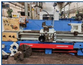
ZMM XL 610X Heavy Duty Lathe Capacity: 615 x 2000mm / Spindle Bore: 103mm
