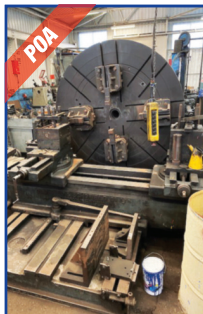
OLDFIELD & SCHOFIELD Facing Lathe. 86in diameter swing
