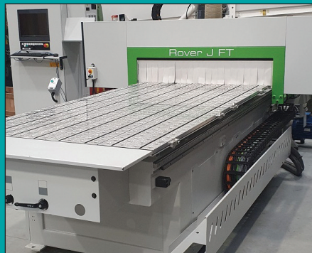
Biesse Rover J FT1224 CNC router, First installed 2019, X=2463 Y=1250 Z=200mm, 22.5 m/min axis speed, spindle speeds to 24000rpm, Biesseworks software £P.O.A.
