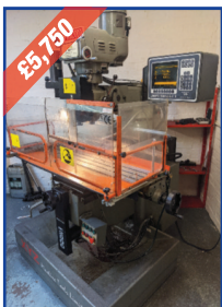
XYZ KRV Pro 2000. 50in x 10in table, R8 taper variable-speed head, ProtoTrak 3-axis control
