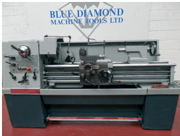
COLCHESTER TRIUMPH 2000 LATHE C/W DRO SYSTEM
