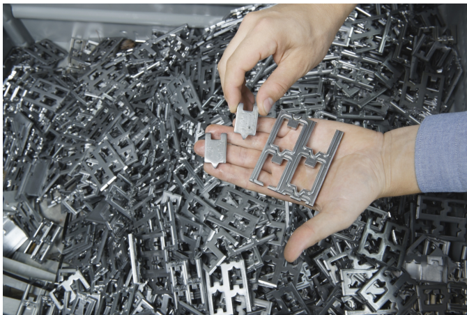
Cut parts and punching waste of test parts with various geometric elements (© WZL)
