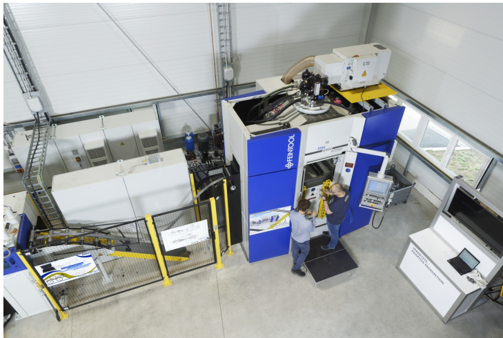
Feintool XFT 2500 speed fineblanking press at the Rotter Bruch site of WZL (© WZL)
