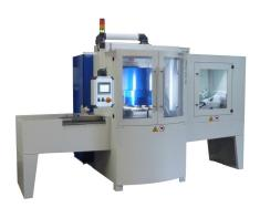
BS Power with its wide belt ensures a high output and processes valve plates that pass through with a diameter of up to  $\emptyset$  400 mm. Its smaller sister, the BS Eco fills the gap as an efficient and cost-effective solution for smaller quantities with a diameter of up to 250 mm.
