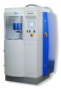
The handling of the BP-MX by touch panel is fast, simple and perfectly controllable. Thanks to the exchangeable revolving or rotary table for rotating parts, the modular machine is available in a user-specific configuration. Tables can be equipped with fixed or swivelling spindles and with cylindrical or hollow taper shank holders.
