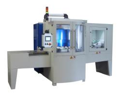
Its smaller sister, the BS Eco fills the gap as an efficient and cost-effective solution for smaller quantities with a diameter of up to 250 mm. The system is compact and reliable and optimally combines three work steps, selective deburring, edge rounding and surface polishing in one process.
